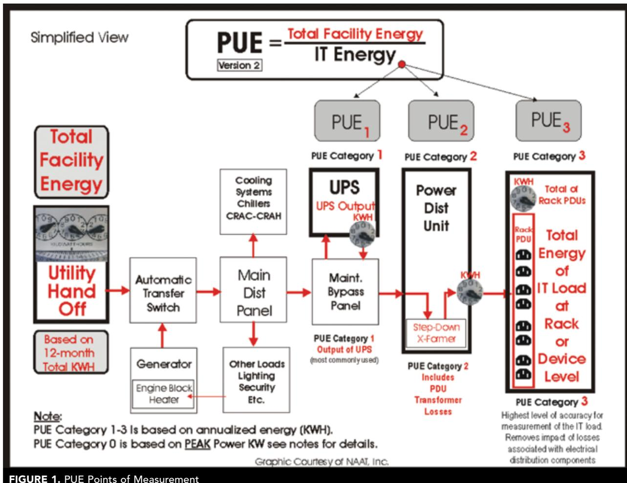
FIGURE 1. PUE Points of Measurement
