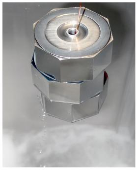
With an eye on their future requirements, NASA tested a number of new solvent choices to compare their clean effectiveness in a vapor degreaser. Here a set of mirrors is cleaned in a vapor degreaser.
