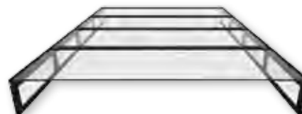
By using the roof the cold air is “trapped” in the contained aisle, the roof also efficiently blocks the hot air to re-enter the aisle
