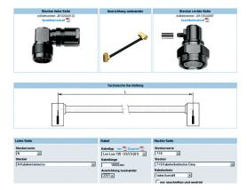
By using Telegärtner's Coax-Configurator, you can design your complete cable assembly, including the connectors, online. Choose from around 400 different connectors and 20 cable types to create your own cable assembly specification which you can download in PDF-format. This specification sheet also shows your individual part-number for the assembly, which you can use to obtain quotations or for ordering purposes.
